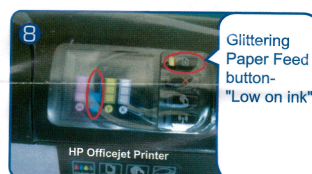
4. The pop-up window "Low on ink" and the low ink column remind you to prepare a replacement cartridge. Or you may judge remaining ink volume by the glittering Paper Feed button and volume indicator as well as the glittering Ink indicator.
