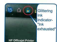
5. Replace the cartridge when "Ink Cartridges Depleted" and "Use Black (or Color) Ink Only?" pop up and the ink column is empty. Or you may judge and replace by empty remaining ink volume and Glittering Ink indicator.
