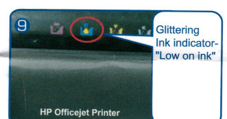
4. The pop-up window "Low on ink" and the low ink column remind you to prepare a replacement cartridge. Or you may judge remaining ink volume by the glittering Paper Feed button and volume indicator as well as the glittering Ink indicator.
